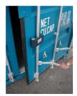
The combination lock can be fastened to the locking bar for storage.
